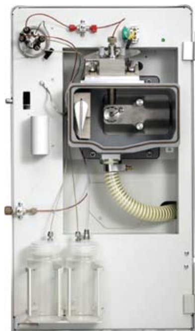
Reference inlet system — calibrant bottles (lower left), flow switching valve (upper left), and source inlet (center).
