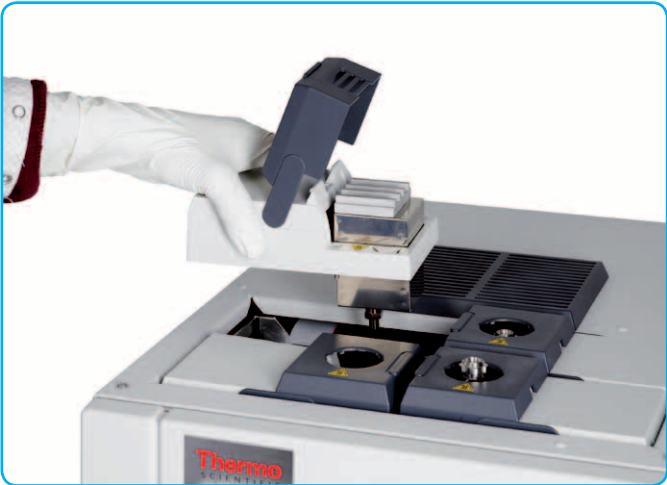
Picture 2. InstantConnect injector, detector and valve technology
