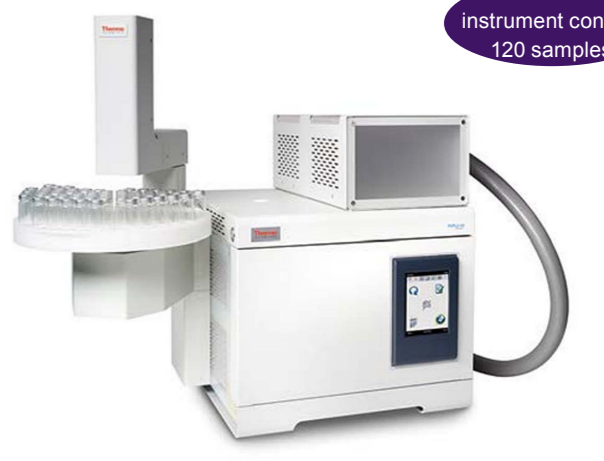
Figure 7: Full instrument control with optional Thermo Triplus 300 headspace autosampler
