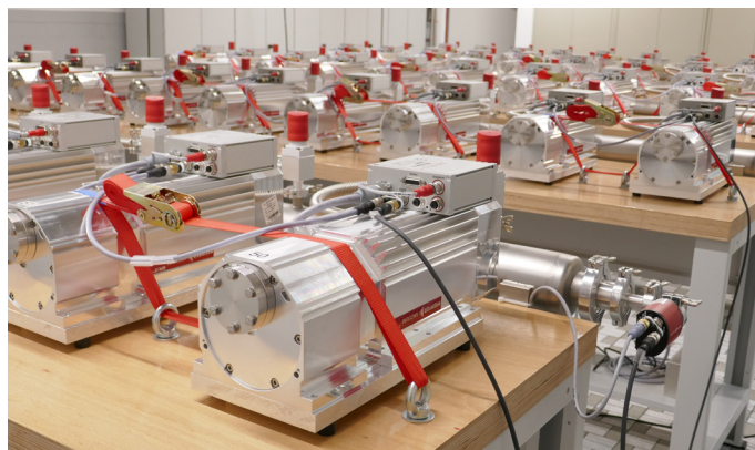
Extensive testing of hardware components, including long-term testing of turbo-pumps
