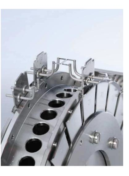
A range of options are available for the Triton XT TIMS. Options for increasing sample throughput include a preheat device for advanced heating of samples and a cryogenic pump for rapid pump down of the source. Options for improving performance for specific isotopic systems include a gas bleed valve for highest ion yields and a high precision pyrometer for filament temperature control.
