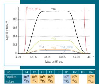
Five  $10^{13}\,\Omega$  amplifiers are recommend for the static Ca measurement as well as a special H4 Faraday cup (requires additional optional items). Peak scan of all Ca isotopes with a cup configuration as shown above of a sample with natural Ca isotope composition.
