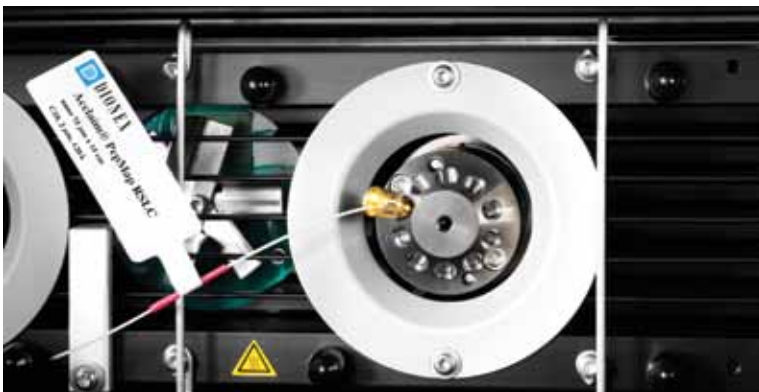
Figure 5. The snap-in switching valve and the proprietary fingertight nanoViper fittings provide the highest level of convenience and confidence for column installation.
