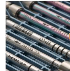
Capped tubes are placed in trays and leak-tested to confirm sample integrity, as required by standard methods.
