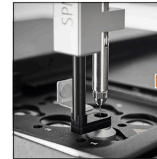
The SPME fiber is positioned in the sample headspace and incubated/agitated to facilitate extraction.
