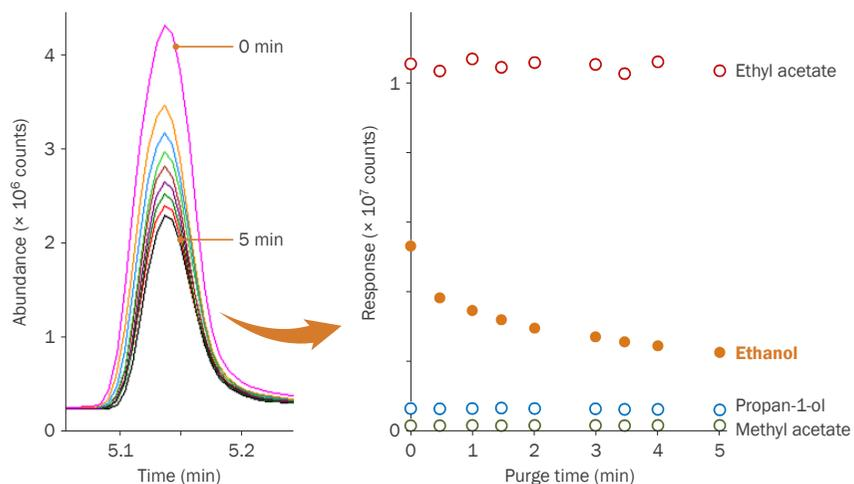
**A significant reduction in the response from ethanol** in this analysis of red wine is achieved by increasing the purge time to 5 minutes. Other volatiles remain unaffected.
