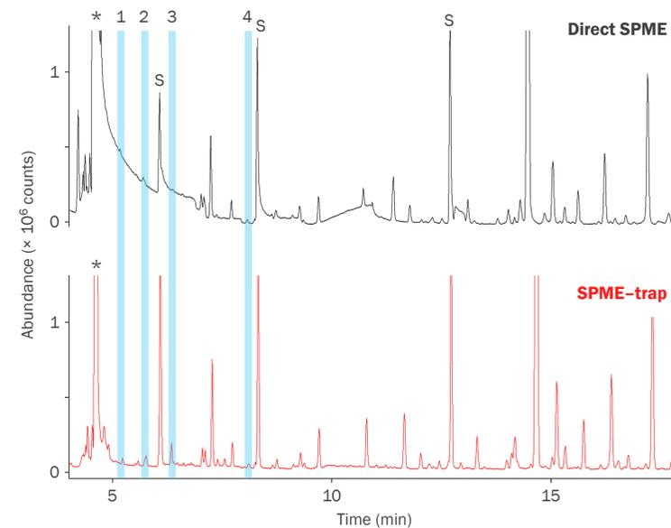
**Improved responses for trace-level species (1-4)** in this tea-leaf suspension are obtained using SPME-trap, thanks to the improved peak shape and a reduced response from diethyl ether (\*), which was previously masking some early-eluting components.
