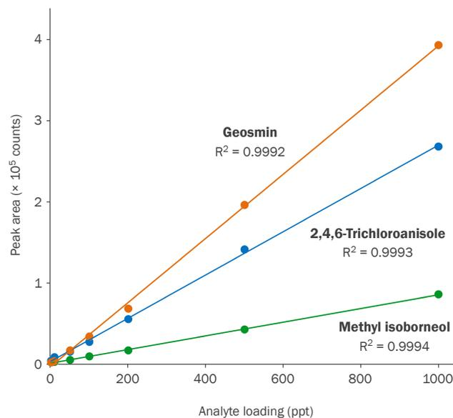
**Excellent linearity from 1 ppt to 1 ppb** is achieved by combining SPME with trap-based focusing for the detection of odorants in drinking water.
