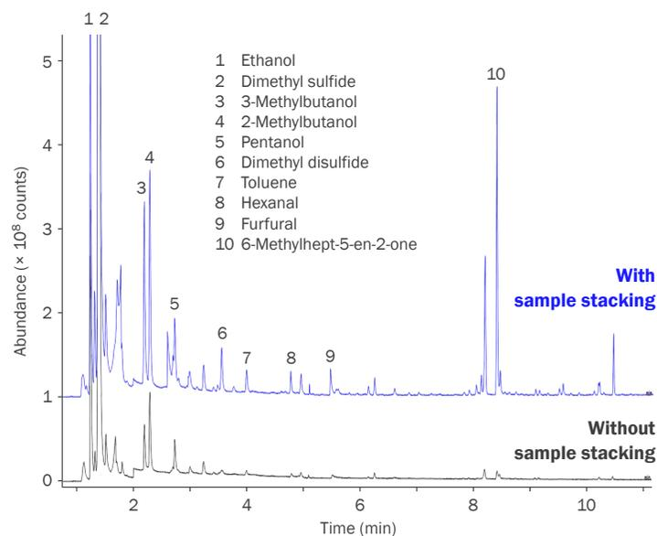
**Trace-level aroma compounds** and contaminants such as toluene were identified in this sample of tomato paste using Centri's focusing trap to boost sensitivity. Stacking multiple 5 mL headspace extractions from the same vial (or different vials) onto the trap further enriches the sample prior to GC injection.
