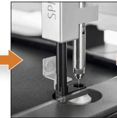
The fiber is inserted into the injection port and the vapours transferred to the focusing trap (or sent directly to the GC-MS).
