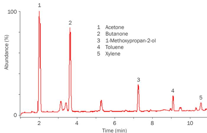
**Off-line sampling of breath** from shoe industry workers, followed by thermal desorption, enables detection of skin-absorbed solvents.
