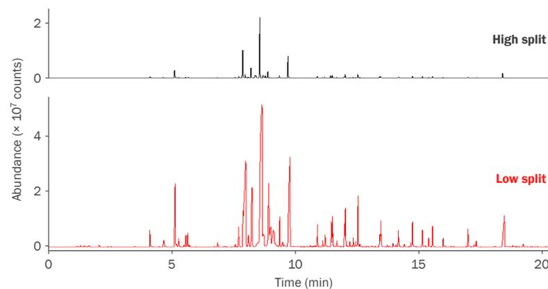
**Re-collection allows multiple methods to be applied to the same sample:** In this example, an initial high split of a candle wax sample avoids the risk of system overload, while a lower split ratio on the re-collected sample allows trace-level components to be detected.
