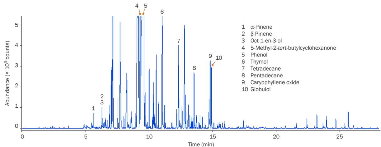
**A range of flavour compounds** are identified in peppermint tea, using direct thermal extraction and TD-GC-MS analysis to generate a comprehensive and representative aroma profile, with no need for sample preparation.
