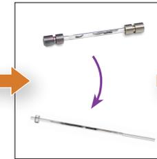
Analytes are released from the tubes in a flow of heated gas, and the vapours collected on the focusing trap.
