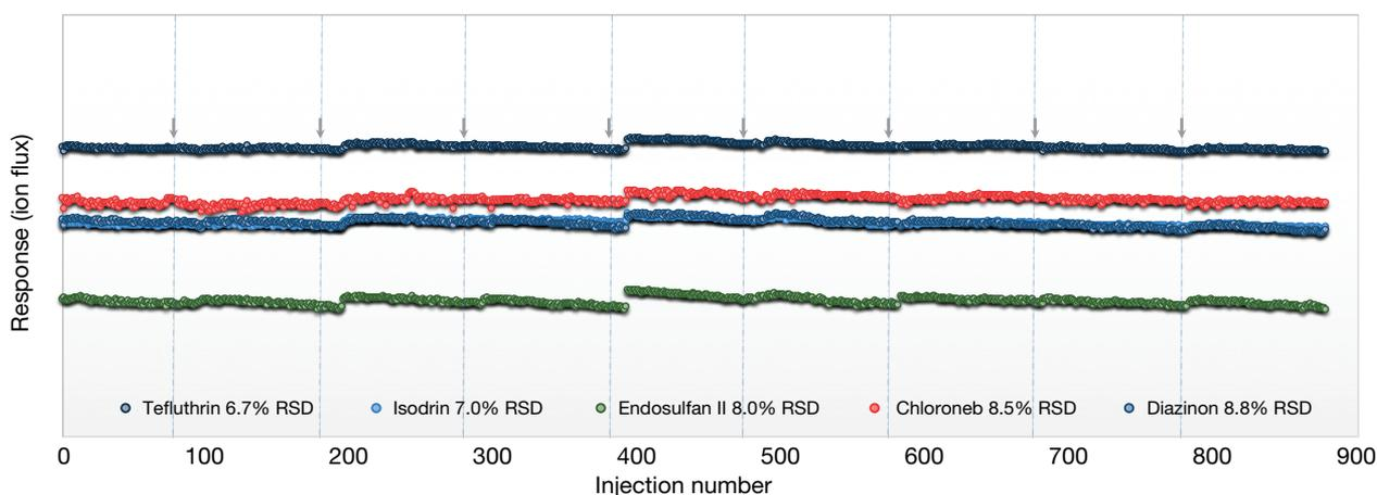
Figure 1. Robustness data showing approximately 900 sequential injections of matrix sample extract spiked with pesticides at 10 ppb [ $\mu\text{g}/\text{kg}$ ]. Injector maintenance and tuning intervals are marked with an arrow. No internal standard correction was used, and no source maintenance was performed during the whole injection series.
