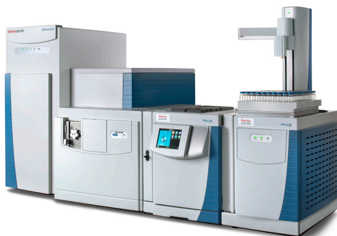
Method parameters: Thermo Scientific Q Exactive GC-MS/MS system coupled with Thermo Scientific TriPlus 500 Headspace Autosampler
