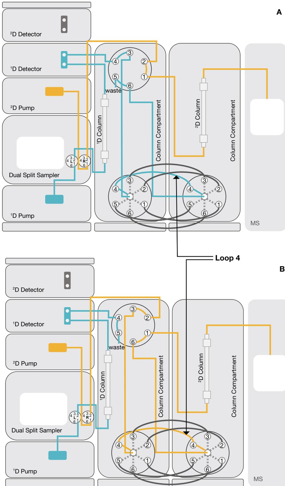
Figure 1. Fluidic configuration of the multiple loop heart-cut 2D-LC system with optional UV as <sup>2</sup>D detector, blue = <sup>1</sup>D flow, yellow = <sup>2</sup>D flow; (A) valve configuration during the <sup>1</sup>D exemplary loading loop 4 (2-p-6-p valve in position 1\_2; both 6-p-7-p valves in position 4); (B) valve configuration during the <sup>2</sup>D analysis of loop 4 (2-p-6-p valve in position 6\_1; both 6-p-7-p valves in position 4)
