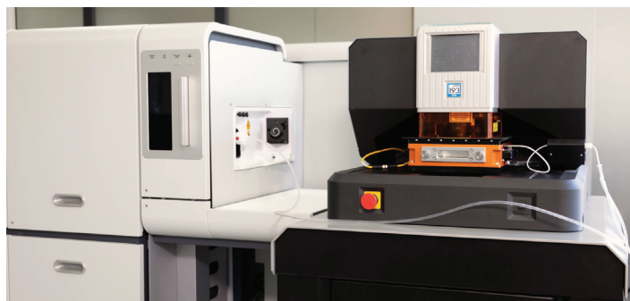
Figure 1. ESL NWR193 laser ablation system coupled to the Neoma MC-ICP-MS
