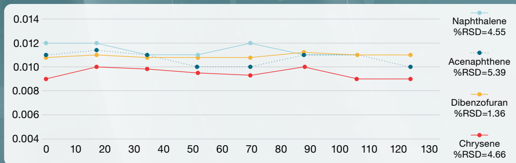
Calculated value of PAHs in QC water at 0.01 ppm over 130 injections
