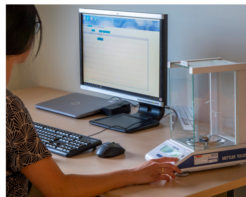
CONNECT A BALANCE TO LABCONNECT AND TRANSFER WEIGHTS FROM THE BALANCE INTO THE FIBERROC AUTO BATCH.
