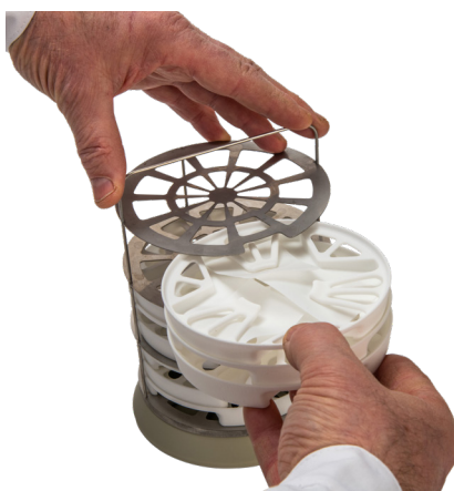
SAMPLE TRAYS AND A SAMPLE RACK MAKES IT EASY TO PREPARE AND INSERT YOUR SAMPLES INTO THE FIBERROC AUTO
